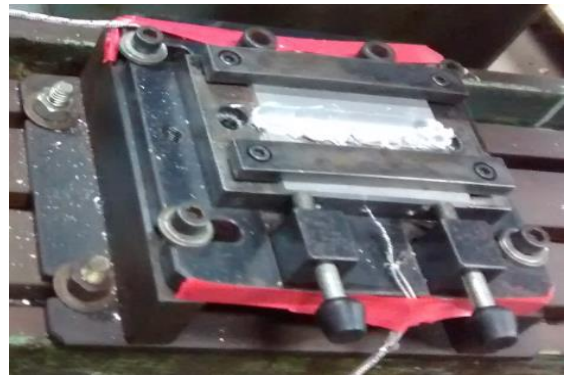
Figure 1 Work Holding setup used for FSW
